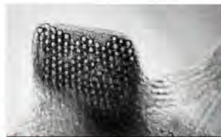
Science 273, 483 (1996) – Crystalline ropes of carbon nanotubes (S. Kim with Nobel laureate R. Smalley)
